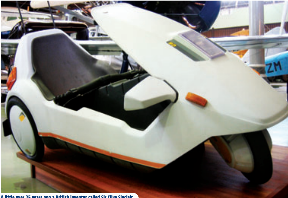
A little over 25 years ago a British inventor called Sir Clive Sinclair invented the Sinclair C5, a three-wheeled electric-powered 'car'.
